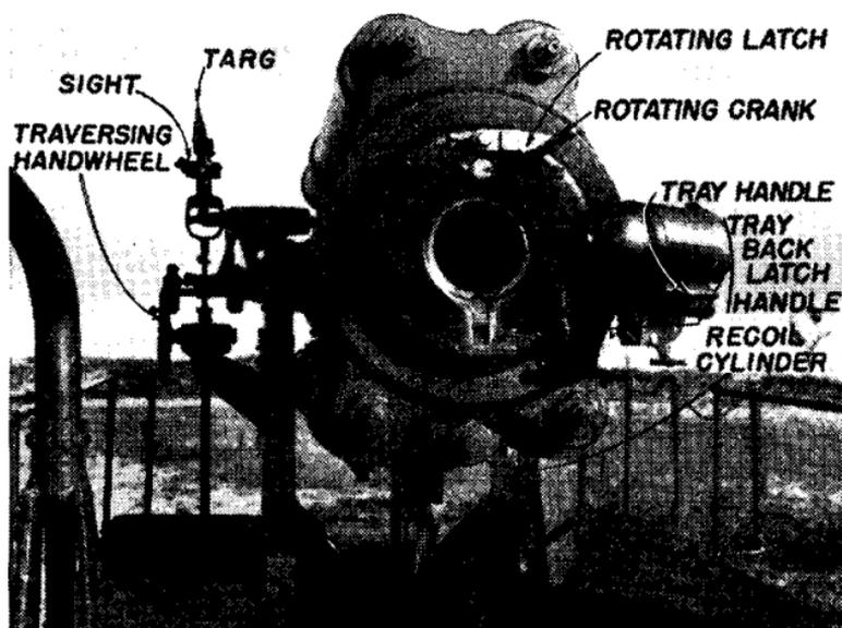
FIGURE 3.—Rear view of 8-inch gun.
