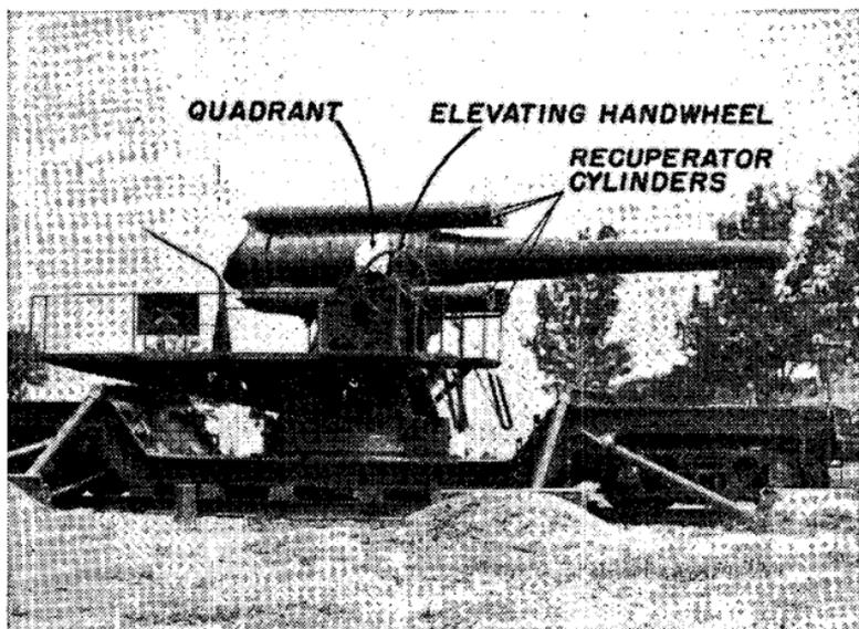
FIGURE 4.—8-inch gun in firing position.
