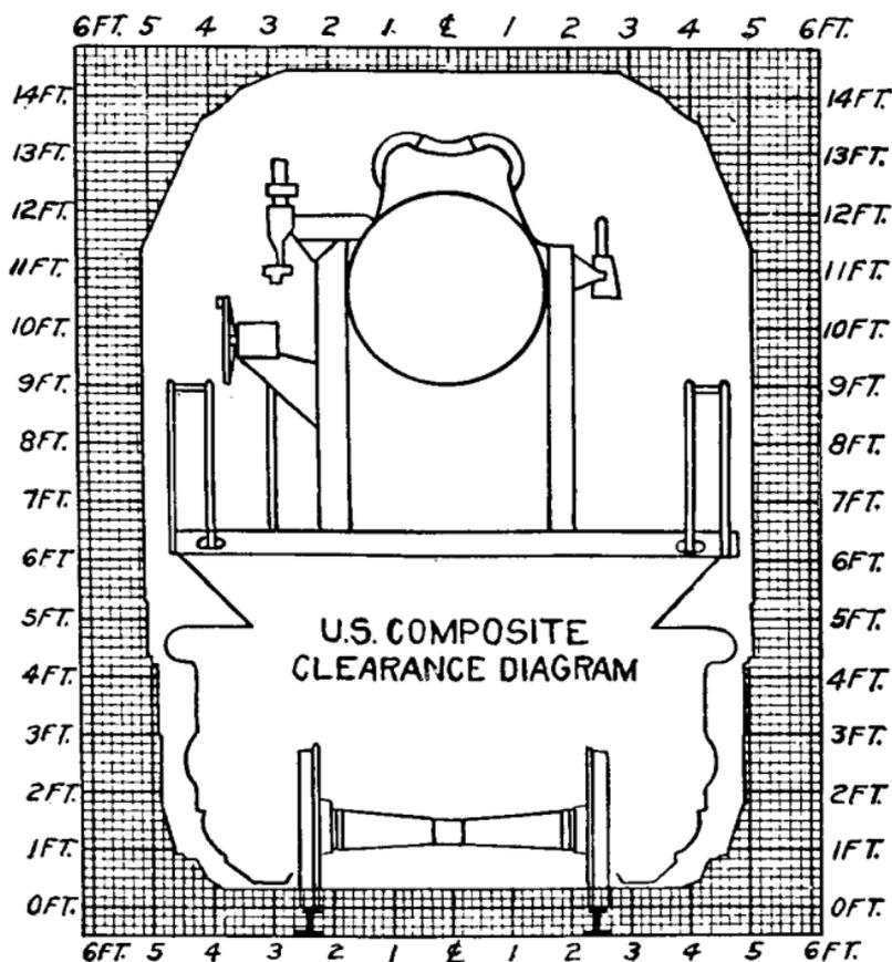
FIGURE 5.—Composite clearance diagram.
