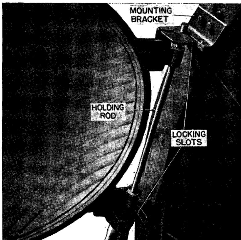
Figure 14. Mounting of spread-beam lenses (upper lens).
