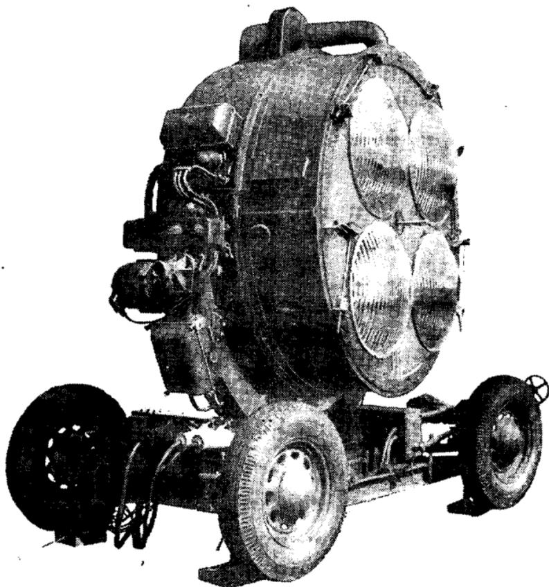
*Figure 6. Searchlight with spread-beam lenses (spread-beam position).*
