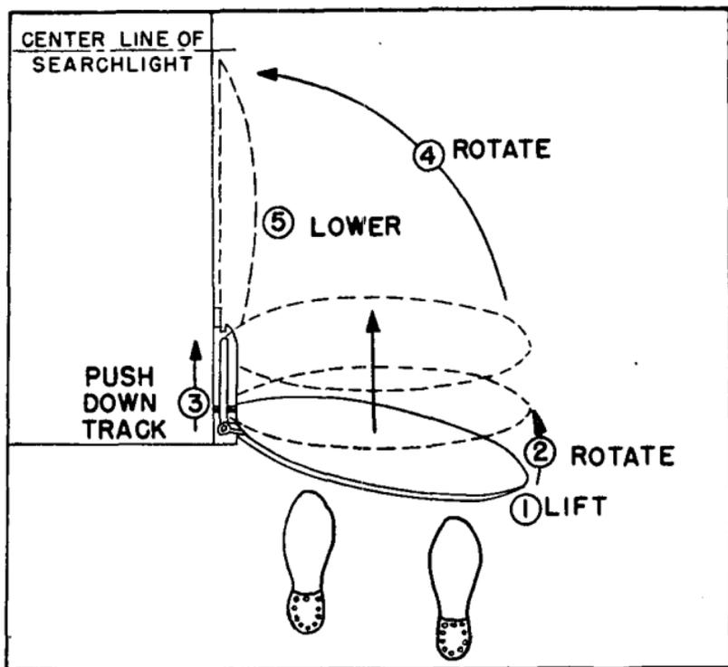
Figure 15. Manipulation of spread-beam lenses.
