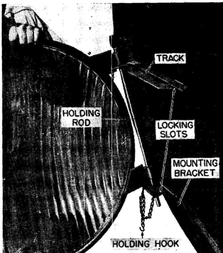
Figure 13. Mounting of spread-beam lenses (lower lens).
